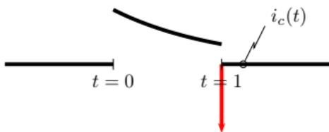
$$\underbrace{i_c(t)}_{=\dot{u}_c(t)} = \begin{cases} 0, & \text{auf } \mathbb{R} \setminus [0, 1) \\ \frac{1}{RC} e^{-\frac{t}{RC}}, & \text{auf } [0, 1) \\ (e^{-\frac{1}{RC}} - 1)\delta_1, & \text{bei } t = 1 \end{cases}$$
