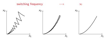
Fixed duty cycle for varying switching frequency (here 45:5555:45)
