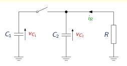
Switch independent:  $0 = v_{C_2} - Ri_R$
